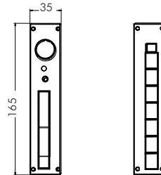
The basic module is the electrical power supply for the light modules. The seven access points or in the back of the module. It is no storage medium or a data processor. It has a integrated serial interface RS232 and can be triggered by a scanner or a system like for example SAP.
